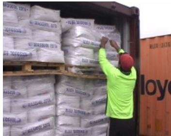
Shrink-wrapping on palletised goods being cut as the goods are loaded into a container before fumigation, to allow penetration of fumigant.
