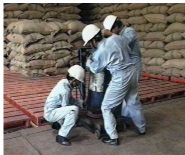
A fumigation team putting a cylinder of methyl bromide on to a platform scale.
